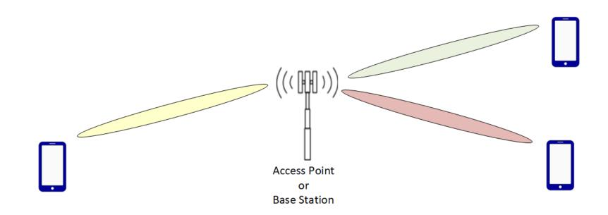
Antenna arrays allow beamforming Beamforming can extend range Multi-User MIMO allows simultaneous connections to multiple users 64T 64R common for 5G, will increase in the future Wi-Fi 7 supports up to 16 antennas
